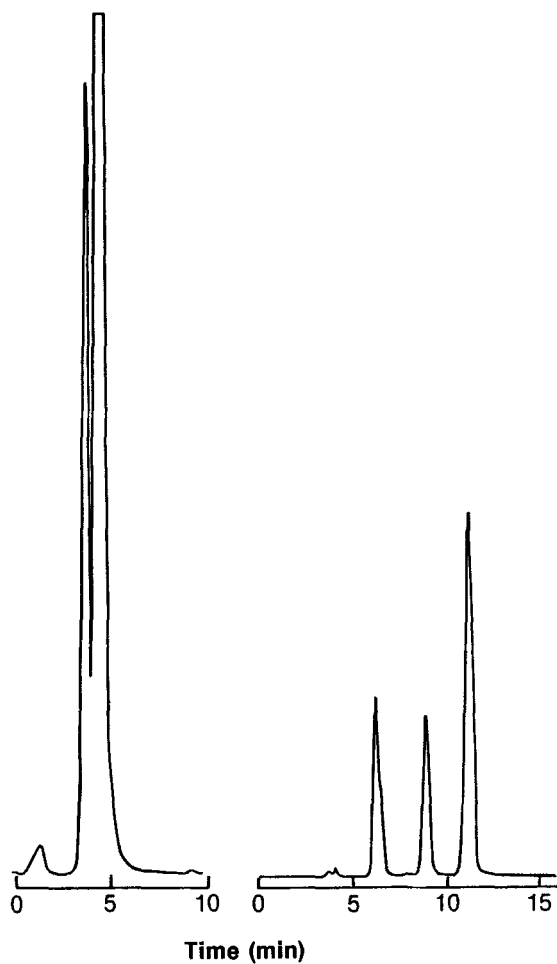
Figure 7. Chromatograms of anticonvulsants using a cation exchange column (left) and a reversed phase C 8 column. The mobile phase used is the same as in Figure 6.
